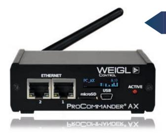
The **ProCommander® AX** is the most advanced micro-sized animation controller ever created, fitting nearly anywhere your attraction requires. Advanced networking with Wi-Fi allows isolated motion and lighting control networks and simplified show system integration. Build shows with full polyphony and thousands of channels of control.
