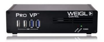
The **Pro VP**<sup>™</sup> is an embedded stand-alone video player solution providing two HDMI outputs, each supporting frame synchronous Full-HD@30fps for 3D cinema projection or simply dual screen. **Pro VP**<sup>™</sup> features Midi and ArtNet time code for synchronizing of external equipment and multi-display solutions. A custom friendly web interface is also provided.
