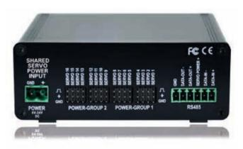
**Pro I/O™** devices deliver many options - analog, digital, relay, DMX-512, CAN, or servo output - to fit your expanding installation requirements in a small, networked form factor. Use any of our familiar software tools for MacOS, PC & iOS to send position commands through a standard control channel.
